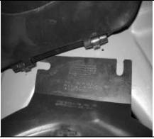
♦Need to reinstall tank / roof screws: Using a 3/8" hex driver for (4) tank screws. Use T-30 torx bit for (3) screws in front left corner of roof & (2) screws in rear left corner of a roof.
